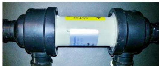
Figure 4: Shell and tube membrane humidifier.
