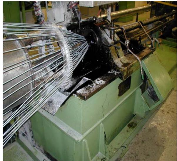
Figure 2: Wires being coated with bitumen
