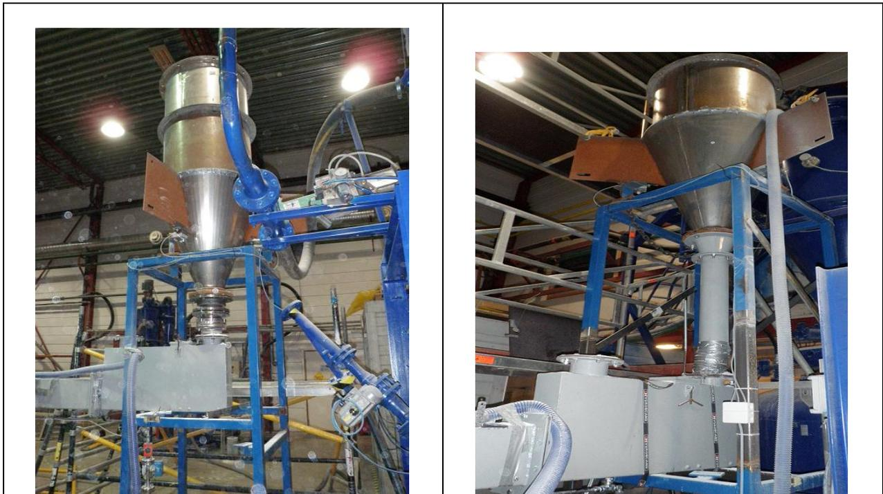
**Figure 1 Experimental setup: a) initial 2012 design using bigger feeding silo, short pipe and iris valve, b) 2013 design using smaller silo, weight beam cells and standpipe concept.**
